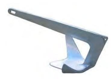
These anchors are not expensive - £44.95 at Force 4 for the 7.5 kg. They work well on a muddy bottom but in Professor Knox's tests the 5kg came up with a holding capacity of 43kgf. He commented as follows: Difficult to engage on hard sea beds. General rating – poor.
