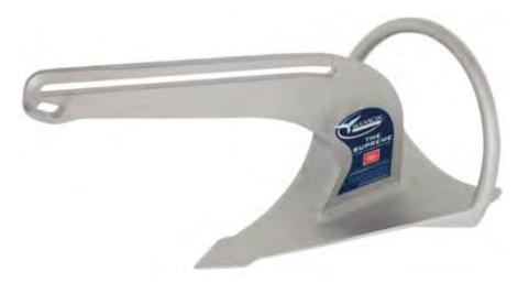
The Manson Supreme is similar to the Rocna, but it has an elongated slot for the shackle onto the anchor chain. This is intended to assist with releasing the anchor if it gets stuck under something. The 7kg version costs £161.99 at Gael Force and has a holding capacity of 90 kgf. It was found to embed immediately and did not break out.
